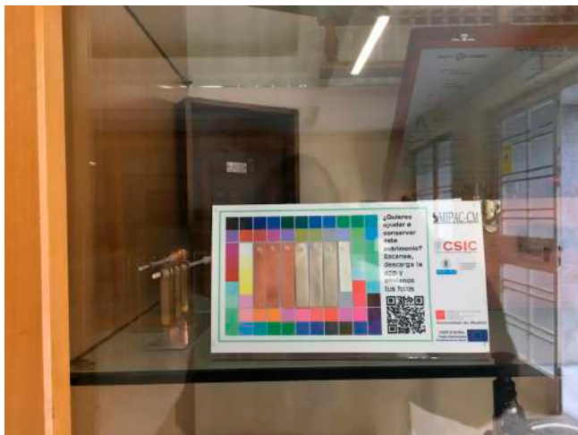
Figure 2. The MIPAC panel monitoring inside a showcase at the Faculty of Chemistry of Complutense University, together with a set of copper and silver coupons on plastic racks (left side)
