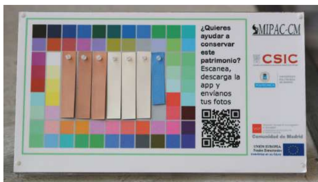
Figure 1. MIPAC panel for the monitoring of color changes of metal coupons. The color chart was printed using UV resistant inks on acid-free paper covered with propylene
